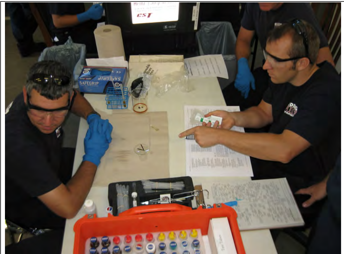
Once again, the team is engaged in Haz Cat operations: the process of identifying unknown chemical substances using chemical ID kits.
